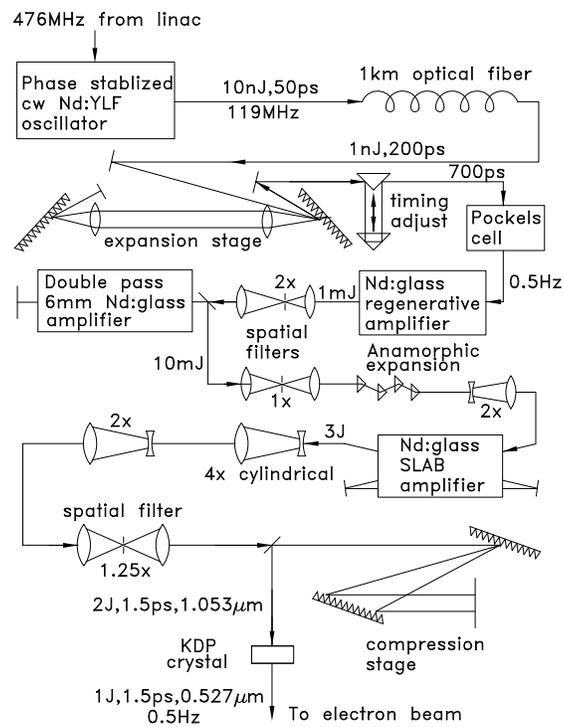
Figure 3: The layout of the E-144 laser system.
