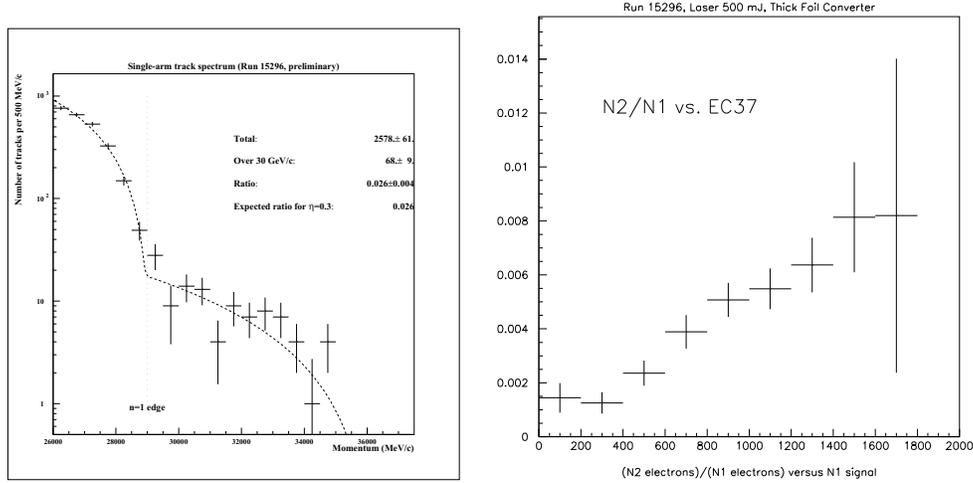
Figure 14: (a) The momentum spectrum of electrons and positrons from conversions of backscattered photons. (b) The ratio of the  $n = 2$  photon rate to the  $n = 1$  photon rate as a function of the latter.
