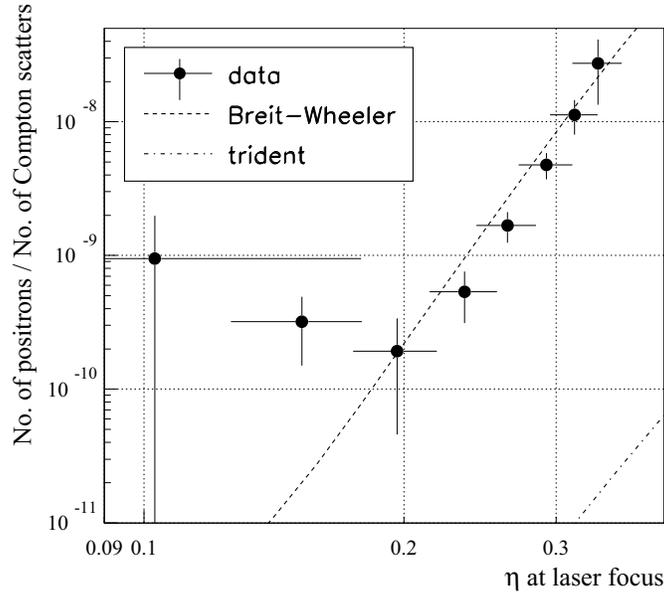
Figure 17: Dependence of the positron rate on the laser field-strength parameter  $\eta$  when the rate is normalized to the number of Compton scatters inferred from the EC37 monitor.
