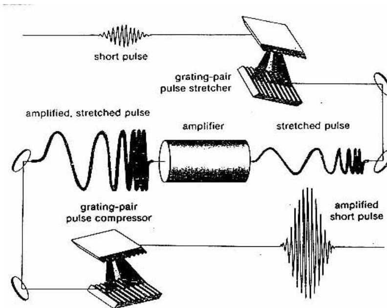
Figure 2: The scheme of chirped-pulse amplification.<sup>19</sup>
