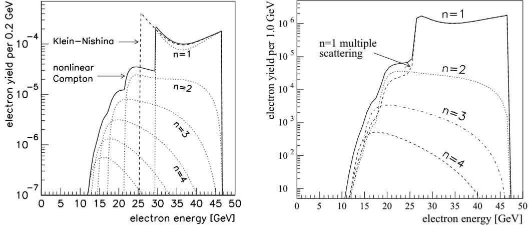
Figure 10: The calculated spectrum of scattered electrons in nonlinear Compton scattering of 46.6-GeV electrons against (a) a 1054-nm plane wave with  $\eta = 0.64$ ; and (b) a 1054-nm laser pulse with  $\eta = 0.64$ , including effects of bunch shape and crossing angle. The yield plotted in (a) is per incident electron; that in (b) is absolute.
