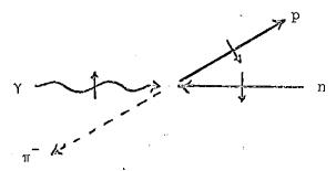
Conservation of parity (and unpolarized initial states) implies the first and third pictures occur equally often, and so the proton spin component in the plane averages to zero. This argument doesn't work for the spin component perpendicular to the plane. Result: in the c.m. frame, any polarization must be in the direction  $\vec{k} \times \vec{p}$  ( $\vec{k} = c.m.$  photon momentum,  $\vec{p} = c.m.$  proton momentum).
