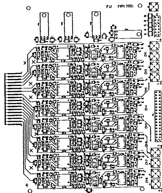
Figure 34: Component layout of the preamplifier card.
