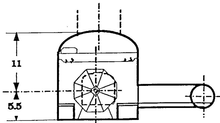
Figure 5.A.2. Interaction Hall Section Without Assembly Hall
