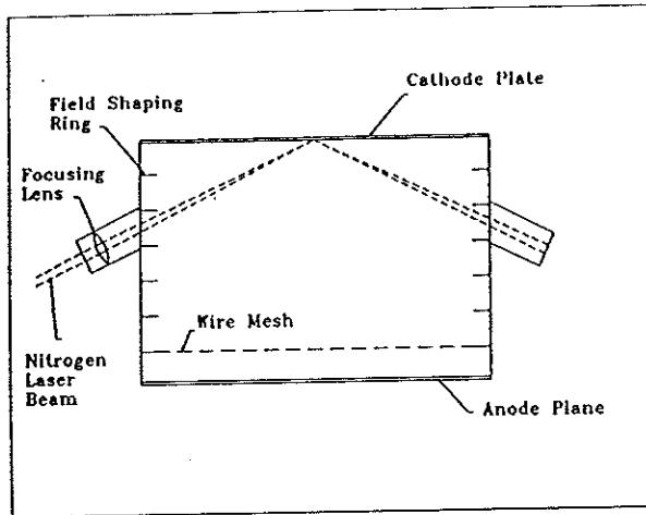
Figure 22: Set-up to measure  $\alpha - \eta$ .
