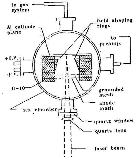
Figure 25: Set-up for measurement of drift velocity.
