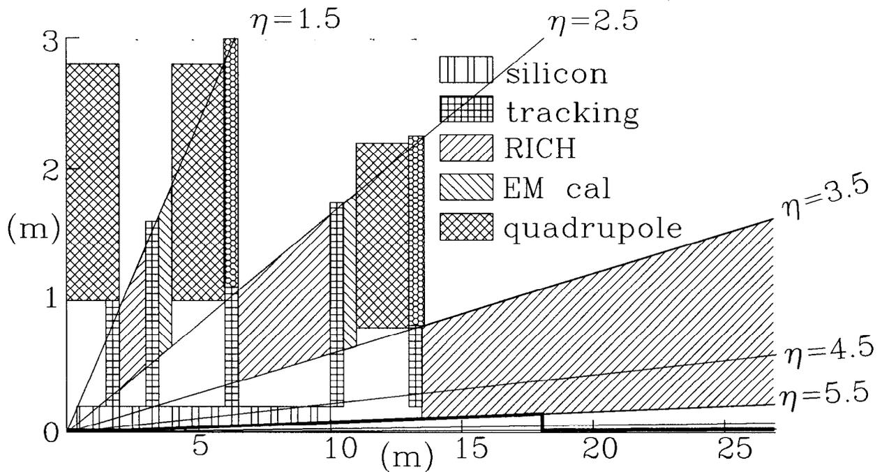
Figure 5: Quarter section of the inner 25 m of a possible first phase of an SSC spectrometer based on quadrupole magnets.
