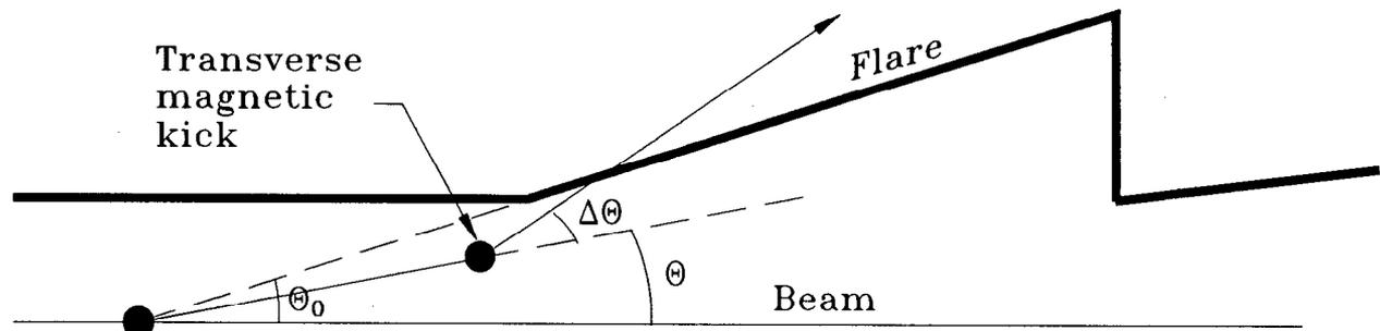
Figure 1: Illustration of how a transverse magnetic field prior to a flare in the beampipe can kick particles into the wall of the flare.
