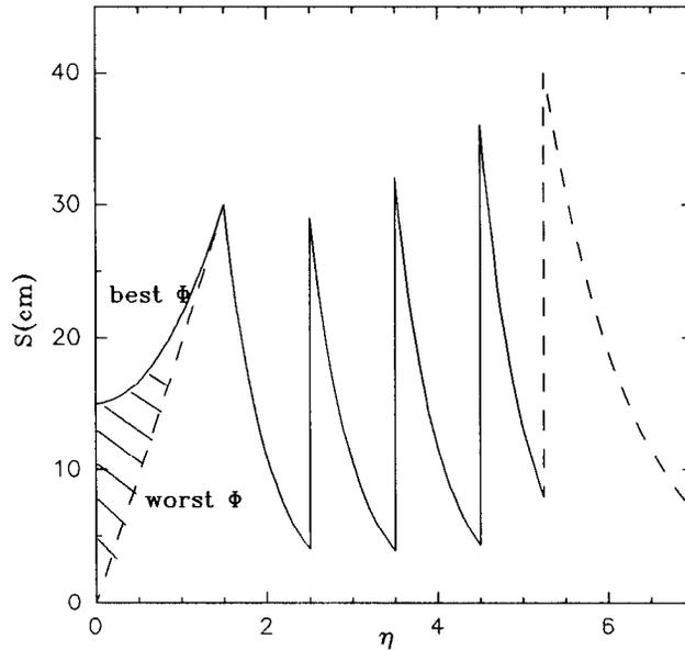
Figure 4: The sagitta as a function of  $\eta$  of charged tracks with  $P_t = 1 \text{ GeV}/c$  that would be observed in the spectrometer of Fig. 3. A dipole magnet is assumed to cover the far-forward region.
