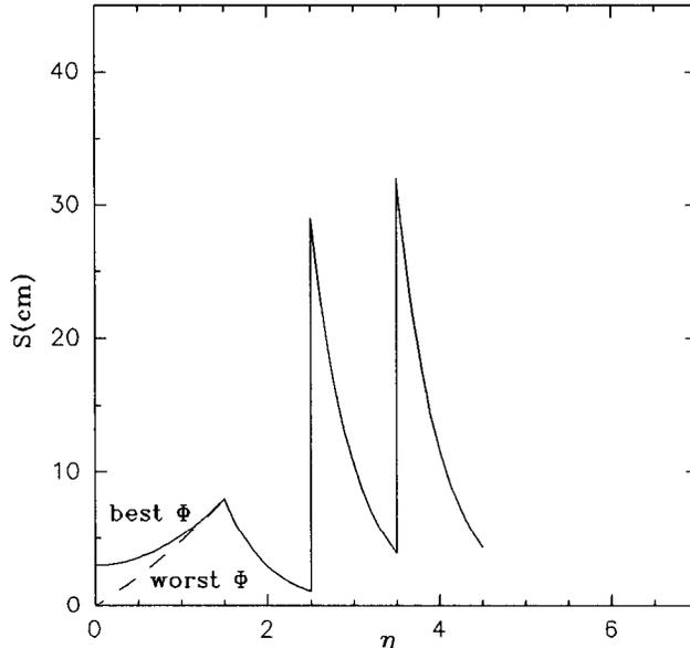
Figure 6: The sagitta of charged tracks with  $P_t = 1 \text{ GeV}/c$  that would be observed in the spectrometer of Fig. 5.
