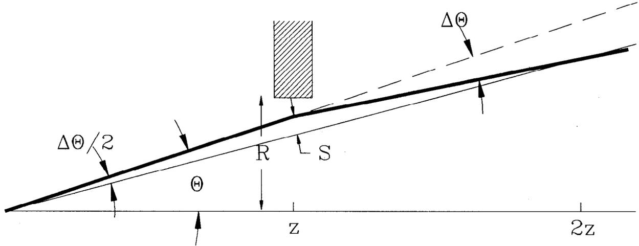
Figure 2: Illustration of the sagitta of the trajectory of a small-angle particle that passes through a forward quadrupole magnet as distance  $z$  for the interaction region. The tracking detectors associated with the quadrupole spectrometer extend out to  $2z$ .
