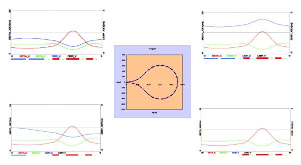
**Figure 47**. The lattice building blocks: triplet 90° phase advance cells; inward and outward cells, missing dipole empty cells.
