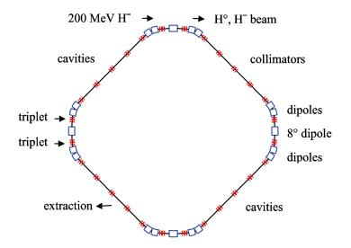
Figure 3. Layout of 50 Hz, 3 GeV booster synchrotron.
