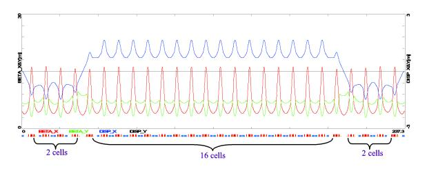
Figure 48. Droplet arc optics, showing uniform periodicity of beta functions and dispersion.
