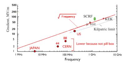
Figure 26. Gradients vs. frequency.
