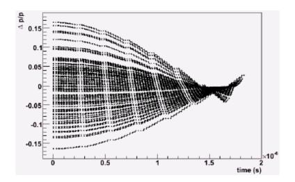
Figure 35. Energy spread of Gaussian beam versus time in the simulation model of PRISM.
