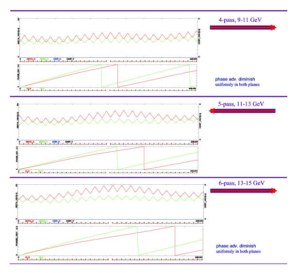
**Figure 46**. FODO based multi-pass linac optics for passes 4–6. Quadrupoles in all cells are set to the same gradient, corresponding to 90° phase advance per cell at 2 GeV. Intrinsic to the FODO focusing symmetry between the horizontal and vertical planes, the betatron phase advances gradually diminish uniformly in both planes. The resulting linac optics is well balanced in terms of Twiss functions and beam envelopes, and there is sufficient phase advance for up to six passes.
