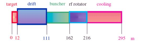
Figure 31. Schematic layout of ISS baseline front end.
