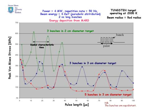
**Figure 15**. Thermal stress as a function of target diameter, number and spacing of proton bunches in a macro-pulse.
