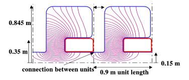
Figure 24. 88 MHz vacuum cavity with integrated solenoids.
