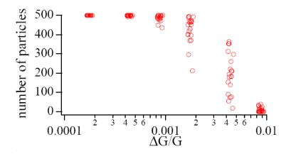
Figure 56. Number of surviving particles as a function of gradient error.
