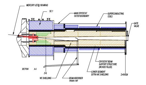
**Figure 18**. Baseline ISS target system. The solenoidal field at the target position is 20 T. The downstream coils begin the process of adiabatically tapering the field to 1.75 T for further transport.
