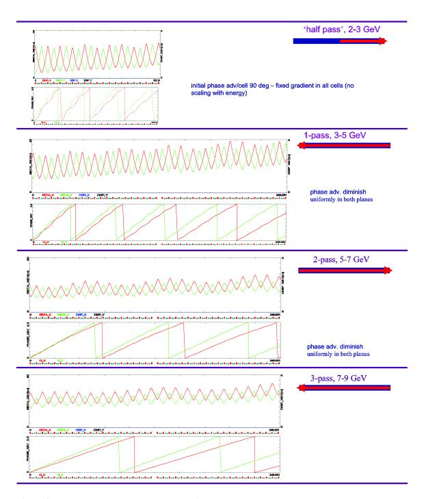
**Figure 45**. FODO based multi-pass linac optics for passes 1–3. Quadrupoles in all cells are set to the same gradient, corresponding to 90° phase advance per cell at 2 GeV. Intrinsic to the FODO focusing symmetry between the horizontal and vertical planes, the betatron phase advances gradually diminish uniformly in both planes. The resulting linac optics is well balanced in terms of Twiss functions and beam envelopes, and there is sufficient phase advance for up to six passes.
