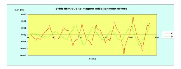
Figure 51. Orbit deviation due to magnet misalignment errors.
