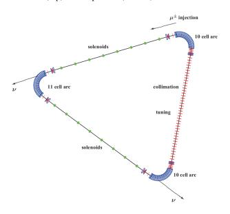
Figure 60. Schematic layout for a 52.8° apex angle, isosceles triangle, muon decay ring.
