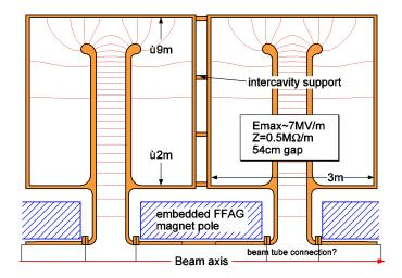
Figure 22. 5 MHz vacuum cavity for FFAG scheme.
