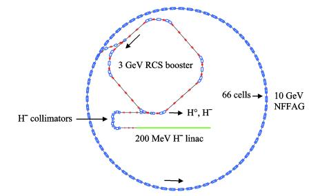
Figure 6. Schematic layout drawing of the linac, booster and NFFAG of the proton driver.
