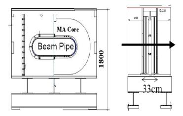
Figure 23. 5 MHz ferrite-loaded cavity for FFAG scheme.
