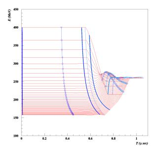
Figure 34. Energy of a set of test particles as a function of time in the phase rotation channel.
