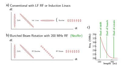
**Figure 19**. Phase rotation methods: a) conventional; b) Neuffer bunched beam phase rotation. c) Shows frequency *vs.* distance for the case of Study 2a, a version of b).
