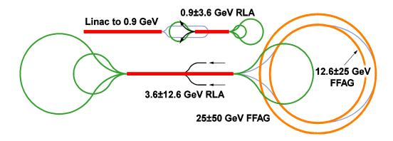
Figure 37. Layout of the acceleration system.
