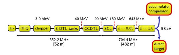
Figure 8. SPL block diagram.
