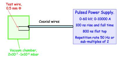
Figure 13. Schematic diagram of the test wire and power supply.
