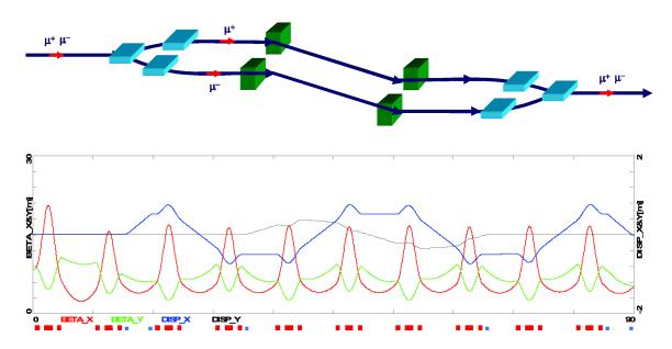
Figure 50. Layout and optics of the injection double chicane.
