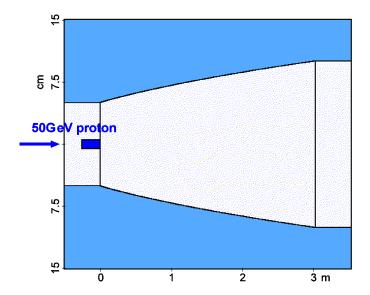
Figure 20. Capture system from ref. [32], comprising a 20 T solenoid followed by a rapid taper to 5 T.
