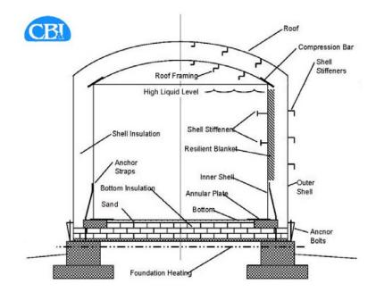
Figure 3: Sketch of a large cryogenic tank designed to contain a liquid-argon TPC (Chicago Bridge and Iron).
