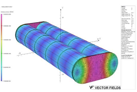
1 m iron wall thickness. ~2.4 T peak field in the iron. Good fielduniformity
