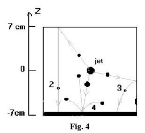
For primary drop radial velocities  $> \sim 1$  m/s, the dominant times involved for secondary drops to clear the collection volume after a beam pulse are the free-fall times for these drops. This is illustrated in fig. 5 for primary drops traveling up with initial velocities of 2.5 m/s, 5 m/s and 10 m/s, stopping at the top and then dropping (case 2, fig. 4).
