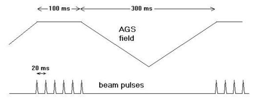
Fig. 1 Proposed beam pulse time sequence
