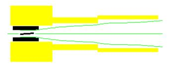
Figure 1: Pion-capture magnet, with average field  $B_0$  in target, -0.3 < z < 0 meters. Magnet mass = 12 metric tons. 4 MW, 21 MJ outer set of coils energizes inner coil. Bore is ~0.15 m near target, ~0.6 m at mouth, z=L. For 0 < z < L, the field profile ramps downward as  $B_0/(1+z/L)$ . The cone is the envelope of captured mesons.
