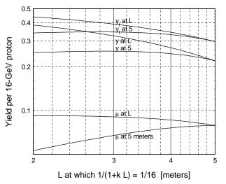
Figure 4: Meson yield per 16-GeV proton. Beam:  $\sigma_x = \sigma_y = 4$ mm. Target: Hg, 20 mm dia. by 0.3 m long, tilted 50 mr.  $y = \pi + K$ ;  $y_t = y + \mu$ .
