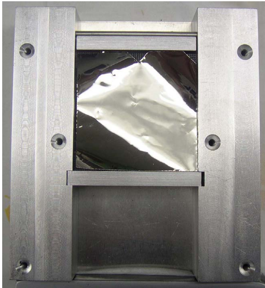
Fig. 6 The nickel foil in the third “basket” of samples that was inserted into the 100-200 MeV proton beam at the BLIP Facility of the BNL linac.
