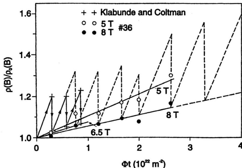
Annealing by cycling to room temperature gives essentially complete recovery of the low-temperature resistivity of Al, but only about 80% recovery for copper.
