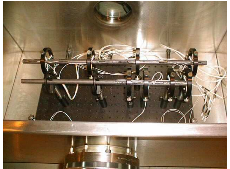
BNL E951 Target Experiment 24 GeV 3.0 e12 proton pulse on Carbon-Carbon and ATJ graphite targets Recorded strain induced by proton pulse
