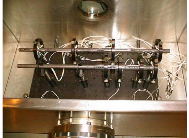
BNL E951 T target Experiment 24 GeV 3.0 e12 proton pulse on Carbon-Carbon and ATJ graphite targets Recorded strain induced by proton pulse
