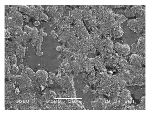
The image above is another 316 steel sample exposed to LBE for 2000 hours at 450 C. X-ray analysis was performed on different, highly localized areas. A quick glance shows that some areas are covered with corrosion, presumably iron oxide.
