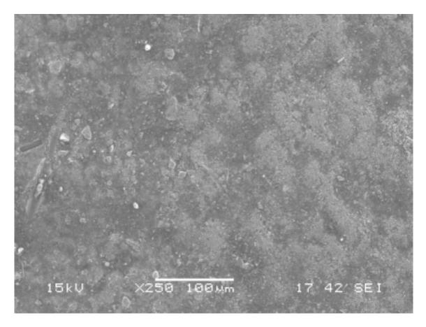
The surface of the exposed, corroded sample is drastically different when viewed at the same magnification.
