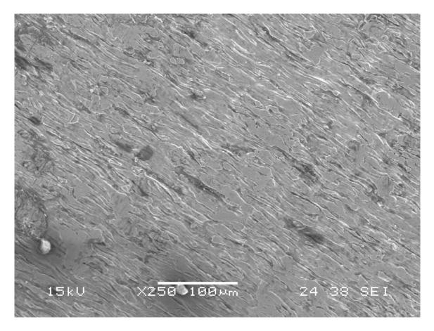
SEM analysis of the surface of the unexposed 316 sample reveals the fresh steel surface before exposure to LBE.
