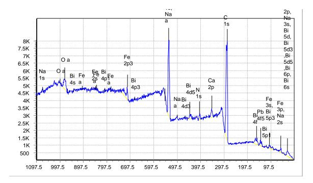
In this spectrum we see the suppression of Cr with respect to Fe as seen in other corroding stainless steel systems. We also see some residual Pb and Bi. Further information can be obtained by looking at peak profiles.
