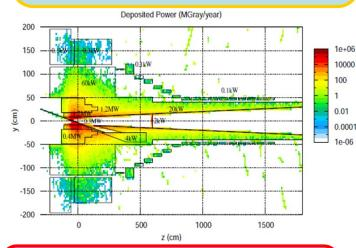
Above: Power deposition in the superconducting magnets and the tungsten-carbide + water shield inside them, according to a FLUKA simulation Approximately 2.4 MW must be dissipated in the shield. Some 800 kW flows out of the target system into the downstream beam-transport elements. See also TUP179.
