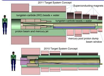
Present concept (top) of a continuous mercury jet target for an intense proton beam. The jet beam is tilted by ~ 70 mrad and with respect to a 20-T solenoid magnet that conducts low-momentum pions into a decay channel. To obtain a 10-year lifetime of the superconducting magnets against radiation damage, a substantial shield of WC beads + water is envisaged. This leads to a much more massive configuration that previously considered (bottom), and a stored magnetic energy of  $\approx 4$  GJ.
