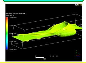
Above: A major challenge is incorporation of the proton beam dump inside the superconducting magnet cryostat. The mercury collection pool can serve as this dump, but the 3-kW mechanical power of the mercury jet will disrupt the pool, unless mitigated by a splash suppressor.
