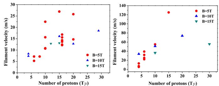
**Extent of the proton-beam-induced disruptions:** Left: the jet disruptions resulting from a 14-GeV proton beam; Right: jet disruptions with a 24-GeV proton beam. In both cases, the proton beam intensity and solenoid magnetic field were varied.
