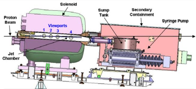
**Cutaway view of the MERIT experiment.** The solenoid/Hg jet system was tilted by 67mrad with respect to the beam/floor. The 15-T magnet was cooled by LN<sub>2</sub> and can be pulsed every 30 min. The hydraulic injection system was capable of delivering an Hg jet of 1-cm in diameter with a velocity up to 20 m/s.
