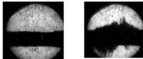
**A proton beam/jet interaction as viewed in viewport 2:** Left image: before interaction; Right image: 500 μs after proton beam arrival.
