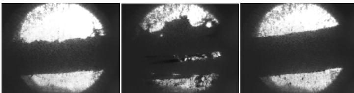
**A proton beam/jet interaction as viewed in viewport 3:** Left image is before interaction, middle image is of the interaction aftermath; the right image is the reformed jet stream.
