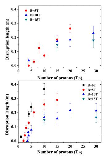
Figure 7: Extent of the proton-beam-induced disruptions: Top: Disruptions resulting from a 14-GeV proton beam; Bottom: Disruptions with a 24-GeV proton beam. In both cases the proton beam intensity and solenoid magnetic field were varied.
