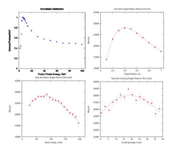
Figure 2: MARS15 simulations to optimize the mercury target geometry.
