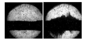
Figure 8: The proton beam/jet interaction of Fig. 6 as viewed in viewport 2: Left: Before interaction; Right:  $350 \mu s$  after proton beam arrival.
