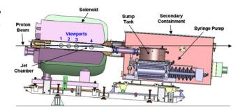
Figure 4: Cutaway side view of the MERIT experiment.
