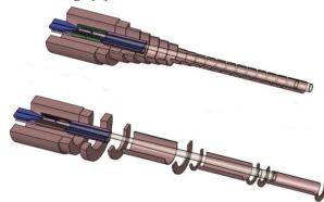
Figure 1: Lower half of the IDS120h (top) and IDS120j (bottom) target system.
