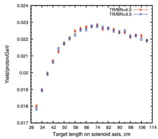
Figure 4: Particle production yields as a function of target length (TR/BR = target radius / beam radius).
