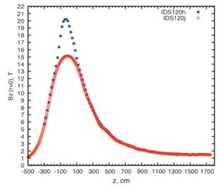
Figure 2: Longitudinal magnetic field along the solenoid axis of SC coils in the IDS120h (dashed line) and IDS120j (solid line) front-end channel.
