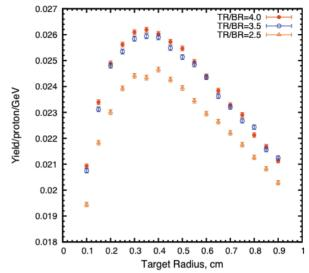
Figure 5: Particle production yields as a function of target radius.
