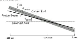
Figure 3: The carbon-target geometry. The proton beam and carbon target cross at z = -37.5 cm. The proton beam is launched at z = -100 cm.
