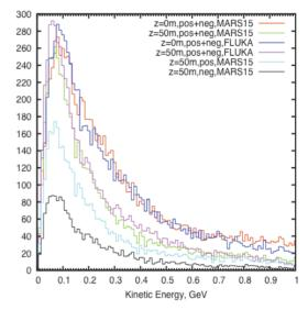
Figure 8: Energy spectra of all positive and negative pions and muons for 3 GeV protons at z = 0 m and z = 50 m for a carbon target from both MARS15 Mode 4 and FLUKA. Energy spectra of positive or negative pions and muons at z = 50 m from MARS15 Mode 4 are also shown.
