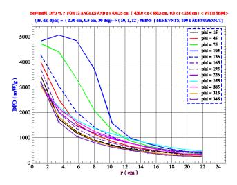
Figure 6: Power Deposition in a 2.5-mm-thick Be window at  $z=430~{\rm cm},$  for 4-MW proton beam power.
