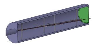
Figure 2: Target vessel with graphite target and proton beam dump. The downstream beam window (green) is of Be.
