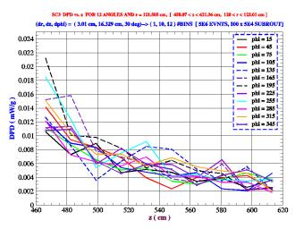
Figure 5: Power deposition in superconducting coil 3 as a function of z, for 12 bins of  $30^{\circ}$  in azimuth, for 4-MW proton beam power.
