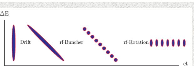
Beam Manipulation: FE manipulates the beam phase-space so that it ready downstream accelerators:
