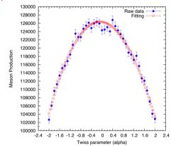
Meson production peaks when the beam focal point is about 5 cm upstream of the beam/jet interaction point, but increase compared to focal point at the interaction point is negligible.
