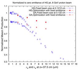
Meson production decreases with increasing proton beam emittance, but careful optimization keeps this decrease to 7% for a Hg-jet target and 4% for a Ga-jet target for a proton beam of 8 GeV kinetic energy and transverse emittance  $\varepsilon$  = 5  $\mu$ mrad, compared to the case of zero emittance beams. The optimized meson production a Ga-jet target is then about 88% of that for a Hg-jet target.
