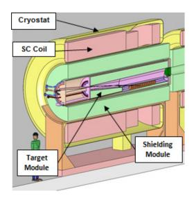
Figure 1: Target cryostat, coils, shielding and Module.
