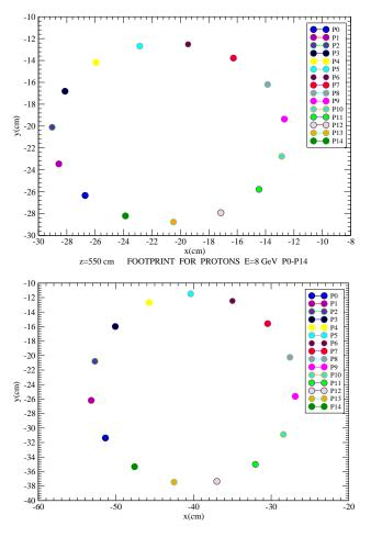
Figure 3: Proton-trajectory intercepts at z = 300 cm (top) and z = 550 cm (bottom) for 15 proton-beam configurations, each of which has the nominal beam/jet crossing angle at the center of the Hg target. The baseline configuration is that labeled P12.
