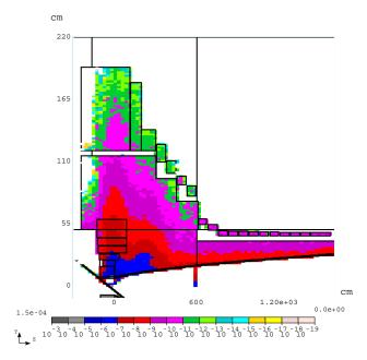
Figure 2: Vertical (y-z) projection of the density (in mW/g) of power deposited in the target region, according to a MARS15 simulation. The peak value in all SC coils is less than 0.045 mW/g.
