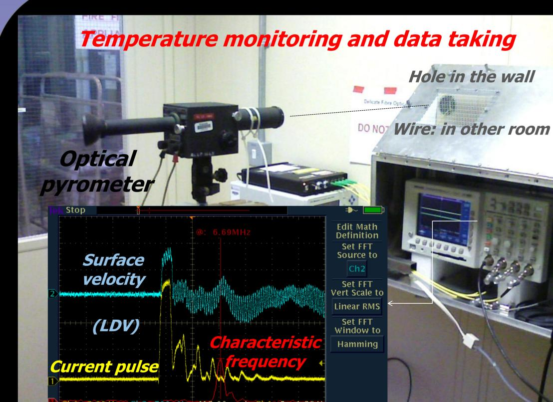
Characteristic frequency of the wire vibration can be used to directly measure Young's modulus of tungsten as a function of temperature.
