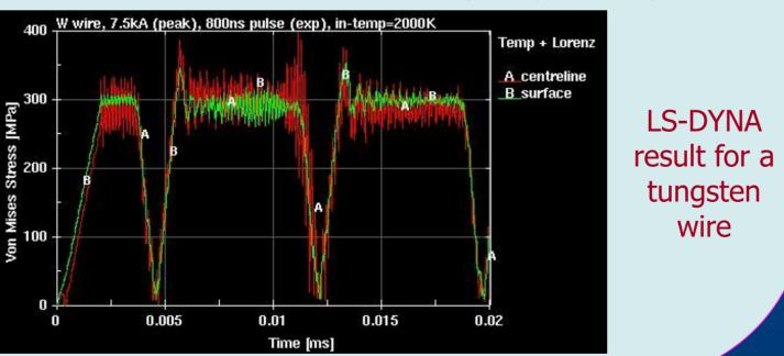
The pulsed heating of a small tungsten (tantalum) wire was proposed as a method for measuring the properties of the candidate materials under controlled laboratory conditions.
