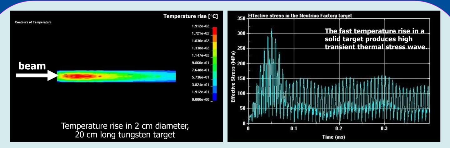
Modern computer codes such as LS-DYNA can be used to simulate the material response in such situations.
