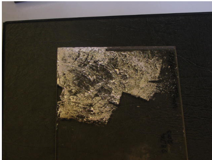
Residue of Belmont alloy 2552 on a quartz window
