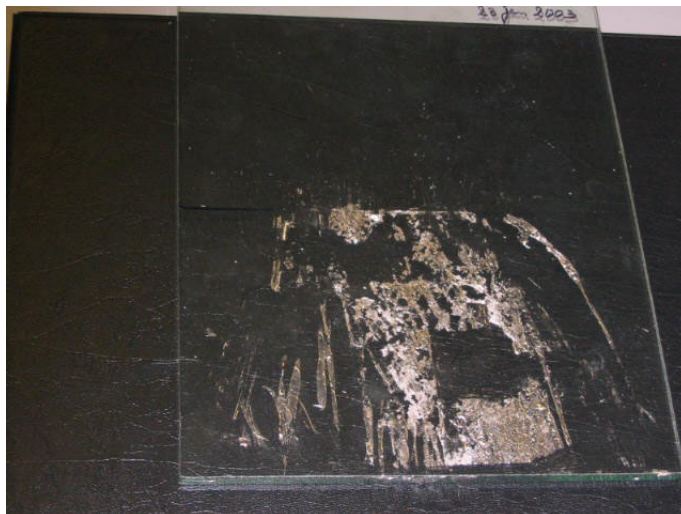
Residue of Belmont alloy 2552 on a glass window
