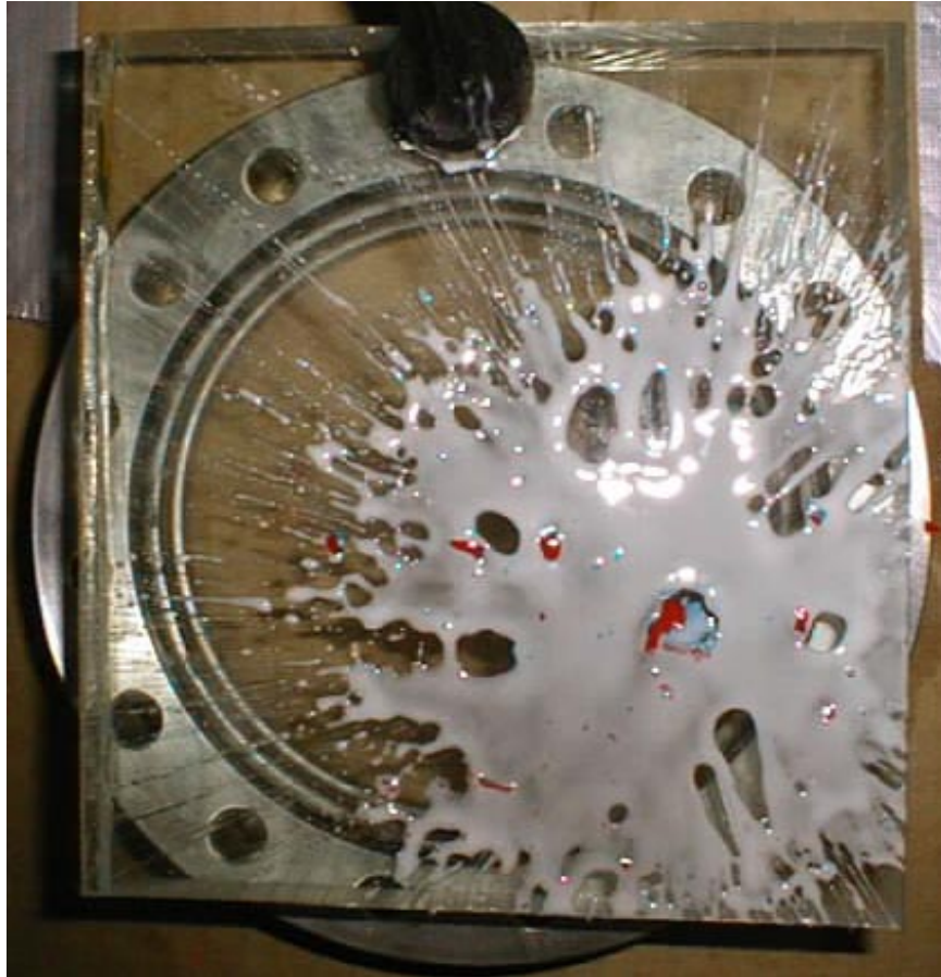
Figure 12: Paintball splat (320 fps) on a 1/4" lexan sheet.
