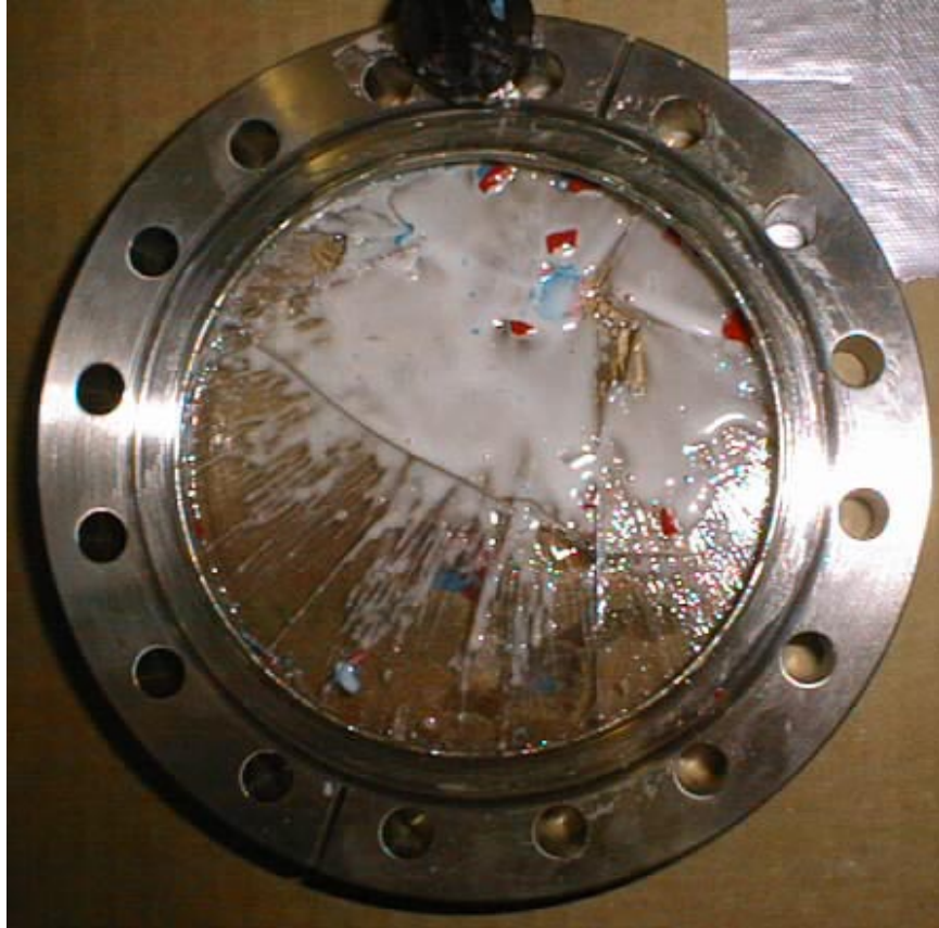
Figure 13: A Paintball splat at 300 fps broke the 1/4" glass window mounted in a 6" conflat flange (MDC Vacuum no. 450006).
