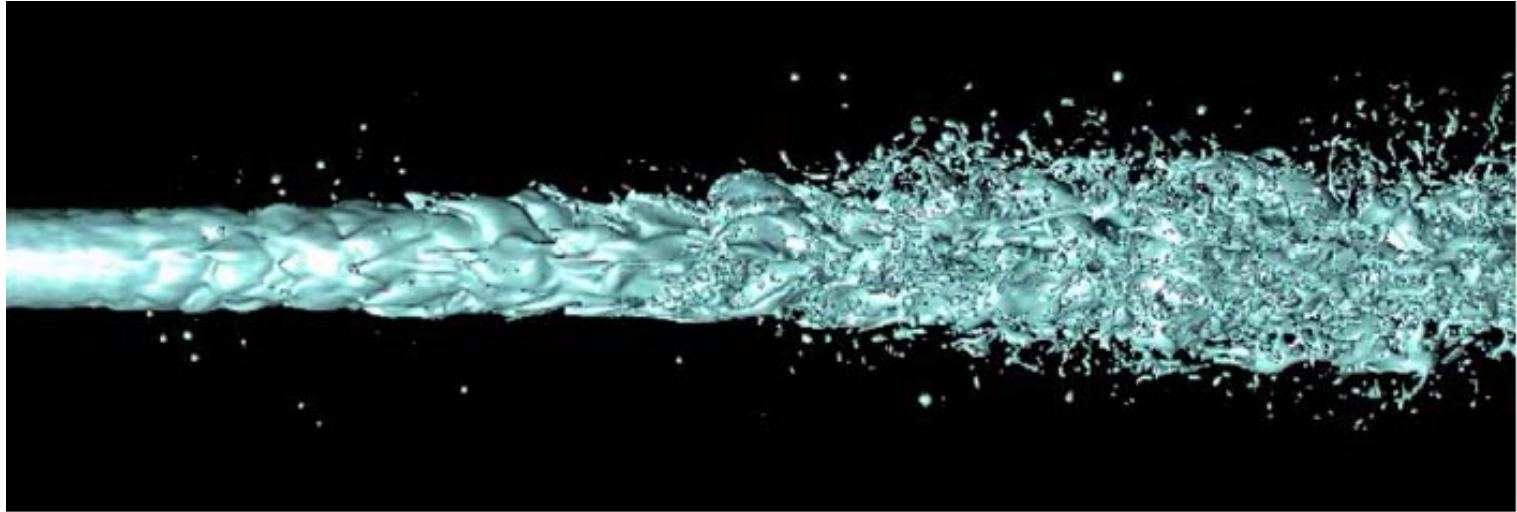
Liquid jet surface and break-up near the jet nozzle
