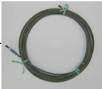
12 meter long, 1-mm diameter BFH37-1000 fiber, blue T=0.77
