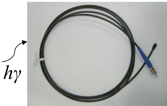
2 meter long, BCF-20, 1-mm diameter blue emitting scintillating fiber
