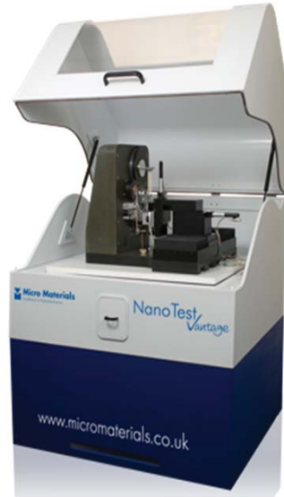
Nanoindenter for micromechanical tests. Plus microscopy
