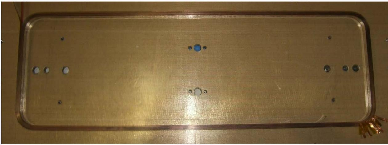
**Partially wound coil with SuperPower tape before the first splice**
