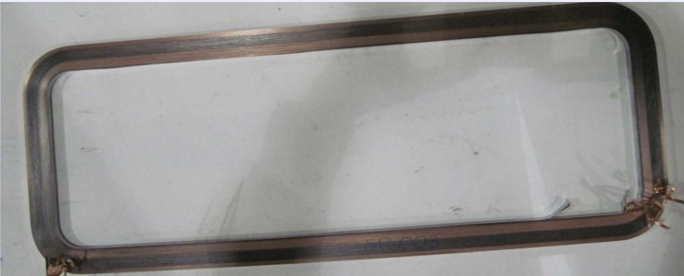
**Fully wound coil with SuperPower tape with one splice**
