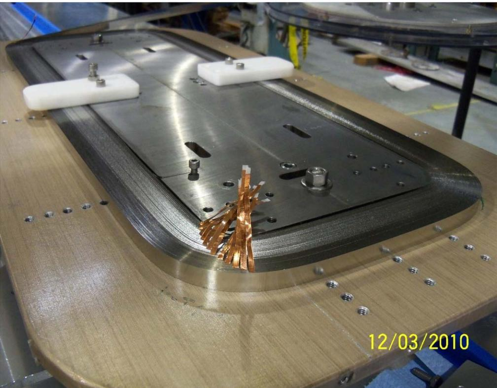
**~210 m (~125 turns), 12 mm double HTS tape per coil.
