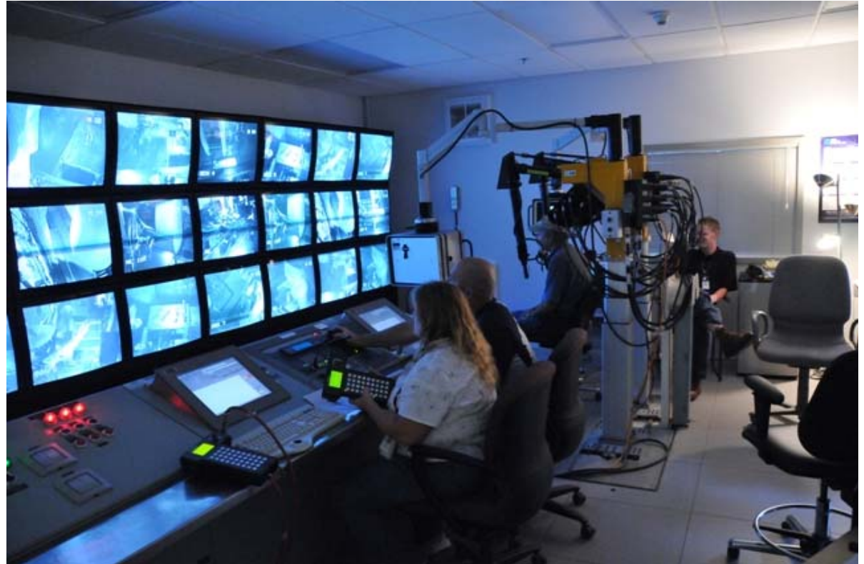
Remote Handling Control Room
