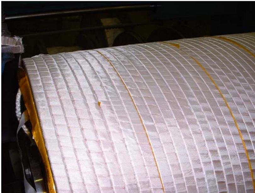
Segment #1 being wound. Photo taken by Dave Rakos at Everson 09-08-04. Kapton layer spaced at every eighth turn relieves axial tension in the layers near the cooling channels. First Layer, Coil Segment#2
