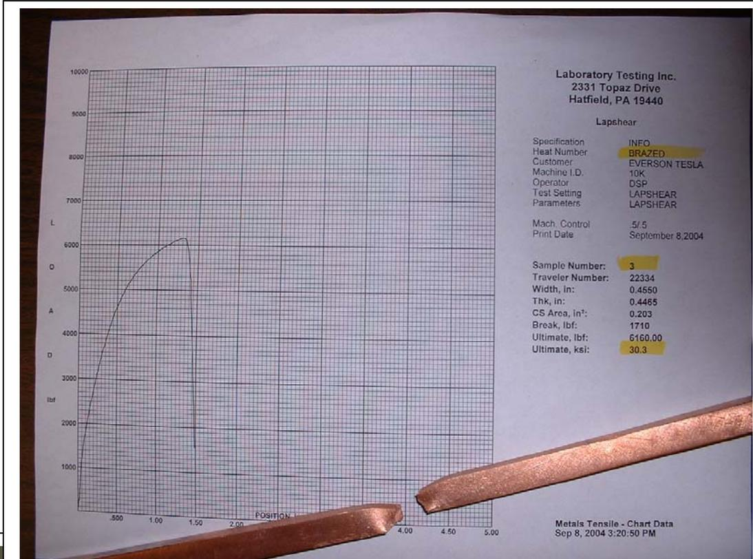
Load Displacement plot of Silver Solder Joint.
