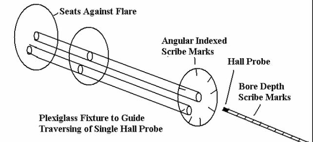
Field Mapping is planned with one Hall Probe at Low Current. Field will scale with current. There are no non-linearities. A Shunt resistor will be used to calibrate CERN power supplies to MIT's
