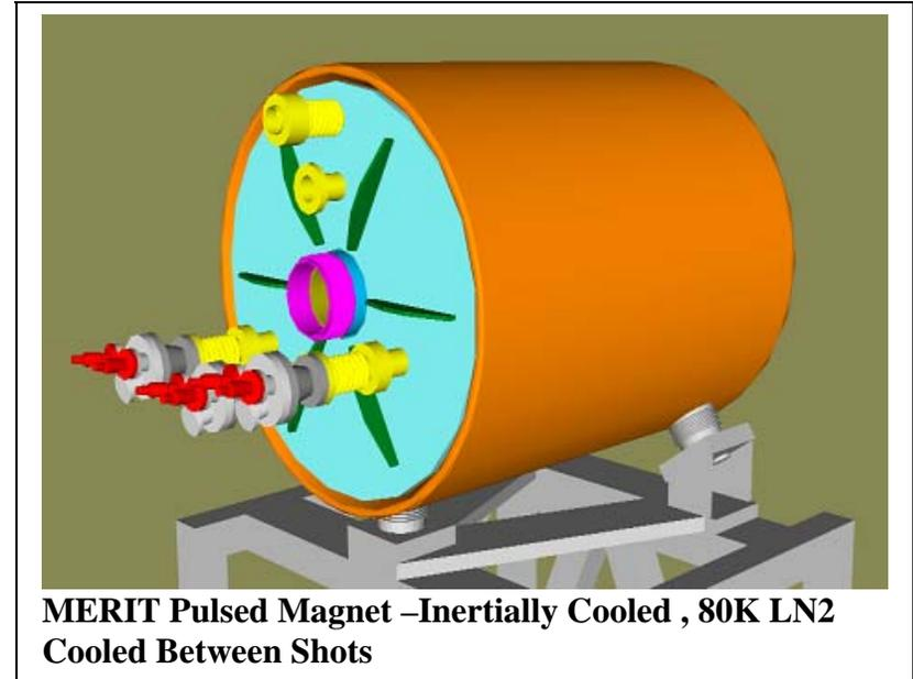
**MERIT Pulsed Magnet –Inertially Cooled , 80K LN2
