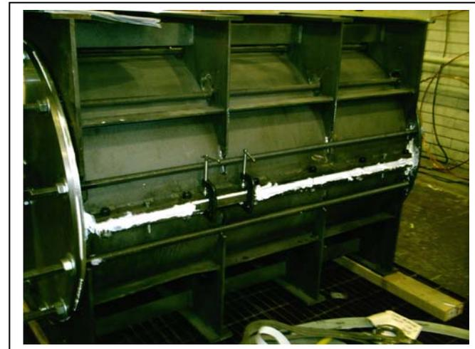
**Segment #3 has Silver Solder Joints and these needed to be qualified prior to winding.**
