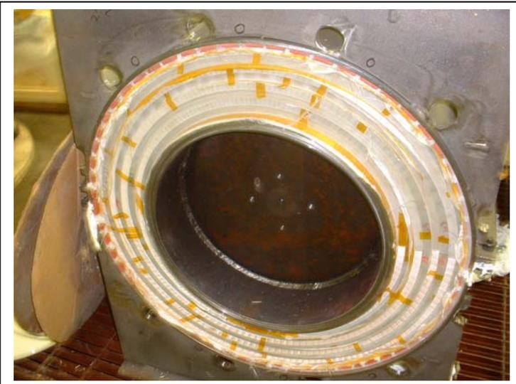
**There was a leak in the longitudinal seam weld. This required application of RTV caulk and additional time to wait for the cure. This was to be held at 2 atm for 12 hrs prior to impregnation**
