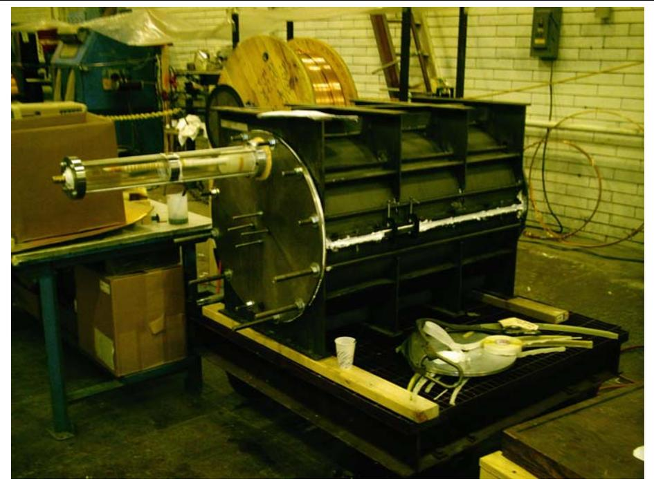
Segment #2 Mold (with Coil enclosed)
