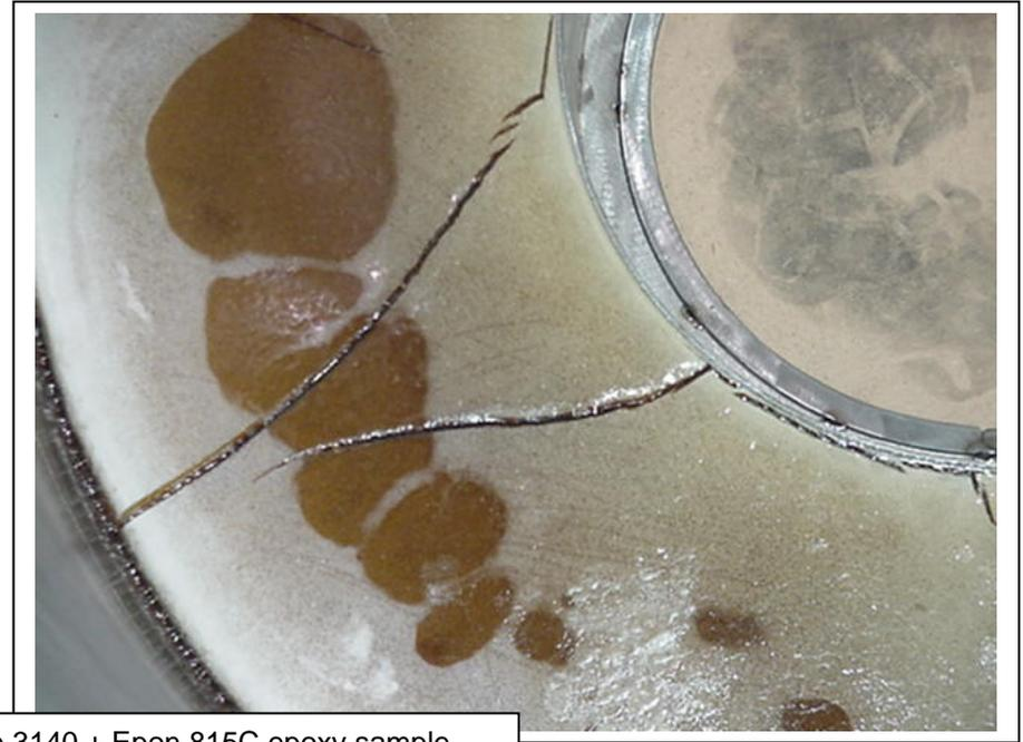
Attached are pictures of Epikure 3140 + Epon 815C epoxy sample. We did not use glass bead as filler because we think it may come loose and damage the valve set of N2 flow control. It's also not recommended by the manufacturer.
