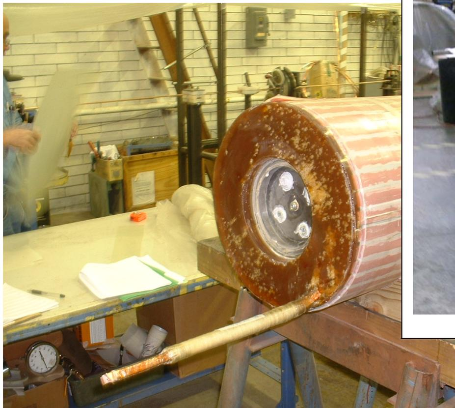
Segment #1 out of the mold. External Silicon fillers that form the “waffle” have not yet been removed
