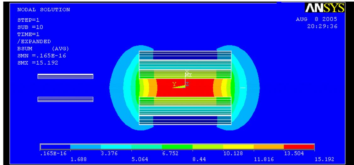
Field Distribution Near the Magnet with a .5 m air gap between magnet and cylinder.
