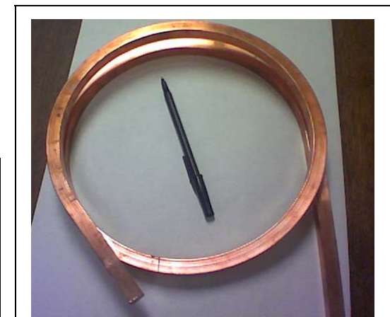
During a March 9 2004 visit to Everson, This preliminary test bend test was shown, and Everson indicated that the keystoneing was “about what was in the spec.”
