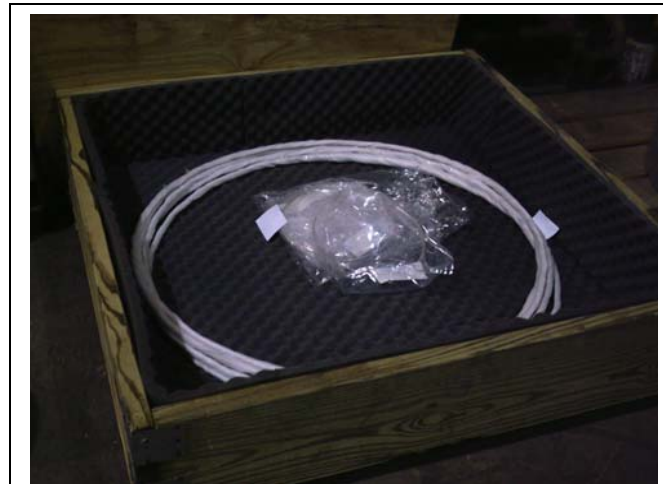
Spare metallic seals for the cover flange
