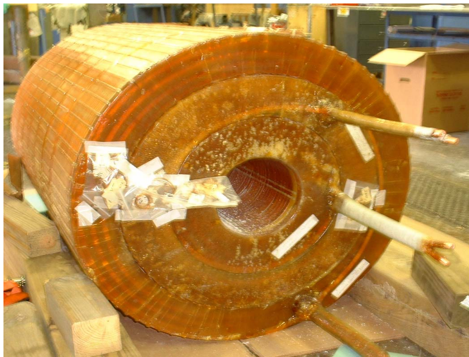
CERNOX Temperature Sensor Leads shown Taped to the Face of the Assembled Magnet
