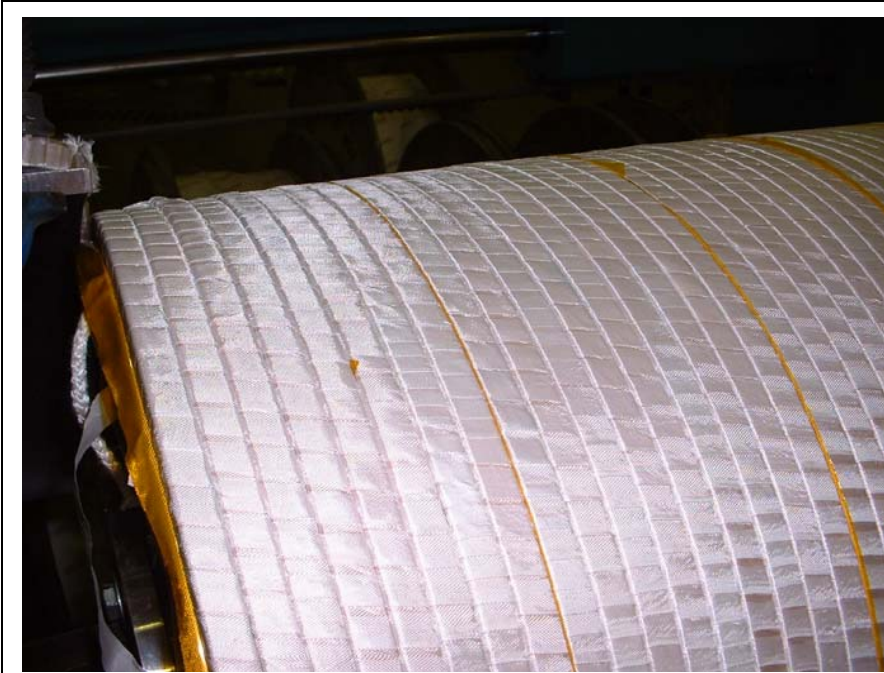
Segment #1 being wound. Photo taken by Dave Rakos at Everson 09-08-04. Kapton layer spaced at every eighth turn relieves axial tension in the layers near the cooling channels. First Layer, Coil Segment#2
