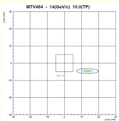
The ellipses indicate the nominal beam position at the flags according to the geometers
