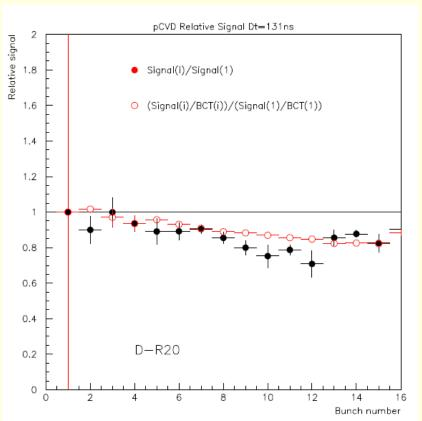
What is plotted is the response per bunch divided by # of protons, normalized to the first bunch
