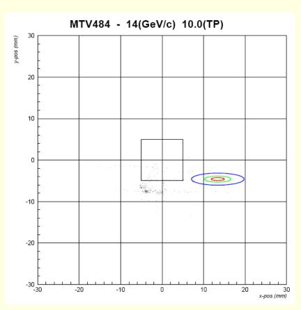
The ellipses indicate the nominal beam position at the flags according to the geometers
