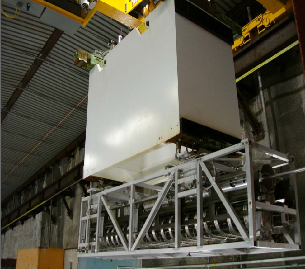
NuMI Low Energy Target and Associated Beamline Positioning Module
