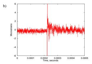
Figure 2: Strain gauge data from carbon targets: a)  $3\times10^{12}$  proton beam on ATJ carbon; b)  $2\times10^{12}$  proton beam on carbon-carbon composite
