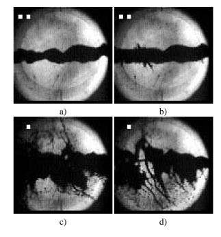
Figure 5: Hg jet interaction with 24 GeV  $3.8 \times 10^{12}$  protons; t = a) 0 ms; b) 0.75 ms; c) 10 ms; d) 18 ms
