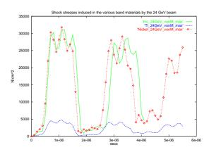
Figure 4: Predicted time dependence of maximum von Mises stresses on inconel 718, titanium alloy and nickel bands due an instantaneous energy deposition from a bunch of  $1.5 \times 10^{14}$  6 GeV protons with transverse dimensions as given in Table 1.
