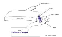
Figure 3: A conceptual illustration of the target cooling setup.
