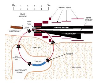
Figure 1: A conceptual illustration of the targetry setup.
