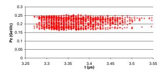
Figure 5. Output bunched beam, capturing from 180<*P*.<230 MeV/c.
