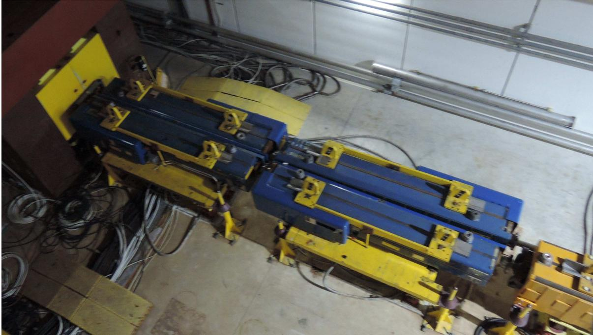
**FIGURE 6.10:** BEND1 and BEND11 in H2 and BEND1 in H4 beam lines in the underground shielded area. The first dipole magnets in the beam lines provide the momentum selection of the secondary beams.
