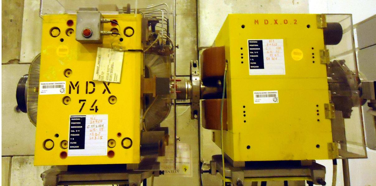
**FIGURE 6.11:** TRIM7 (left) and TRIM8 (right) in H2 beam line serve for fine beam steering in vertical (TRIM7) and horizontal (TRIM8) directions. Note that they are installed around the short vacuum beam pipe; before and after this vacuum section the beam travels through the air.
