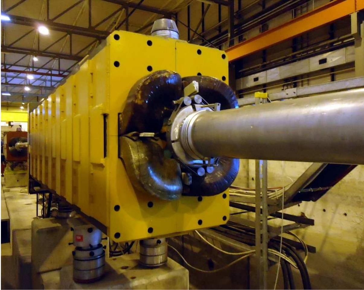
**FIGURE 6.12:** One of the Quadrupole magnets in the H2 beam line. Most frequently used for focusing of the beam on the main experiment, if needed, they can also be used to create quite sophisticated beam profiles.
