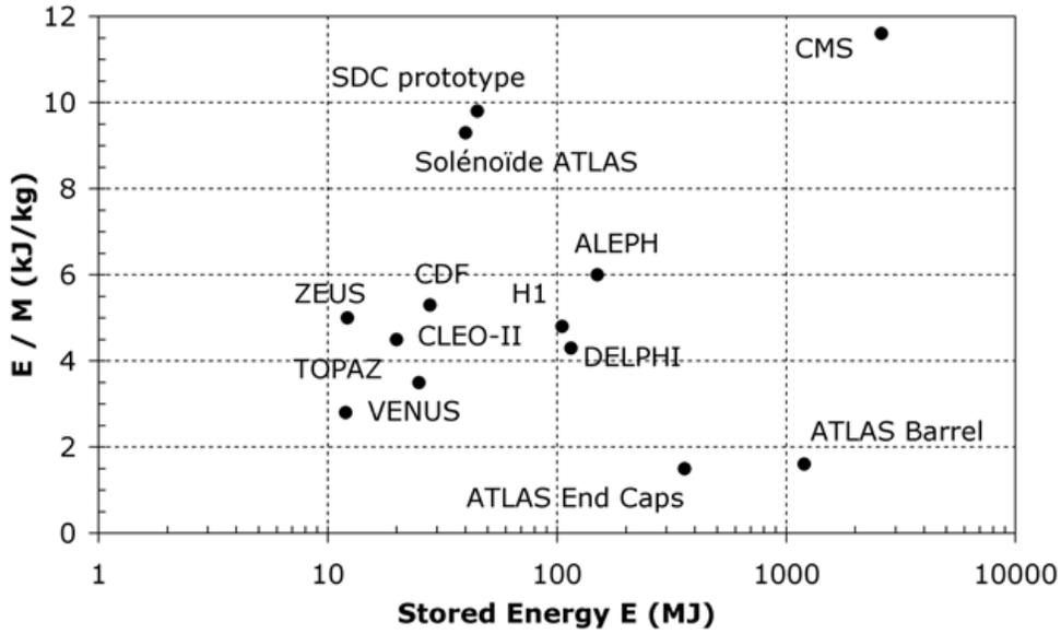
Figure 2.8: Comparison between the CMS solenoid and various other detector magnets. The x-axis (log scale) corresponds to the stored energy,  $E$ , of the magnet in units of MJ. The y-axis corresponds to the ratio between nominal stored energy and nominal effective cold coil mass of the magnet,  $E/M$  in units of kJ/kg. The CMS solenoid surpasses all of the other magnets displayed here with respect to both variables [67].
