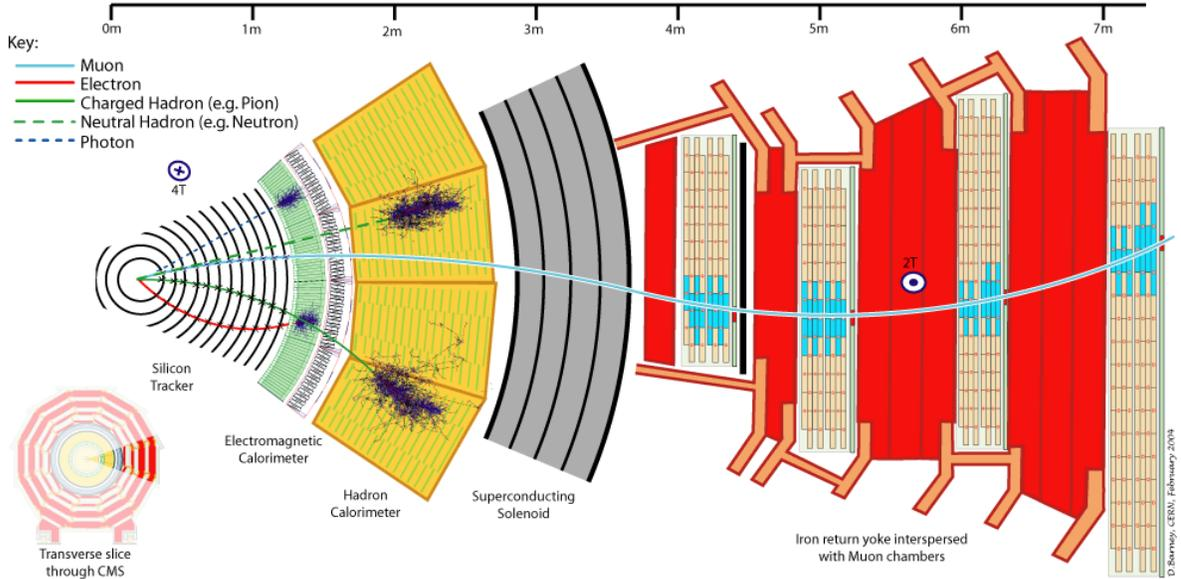
Figure 3.1: A cartoon schematic of the CMS detector, shown in the  $r - \phi$  plane. The ideal interactions of muons, electrons, pions, neutrons, and photons with various components of the detector are shown.
