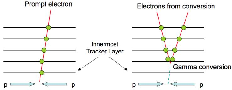
Figure 6.1: Prompt electrons originating from the primary  $pp$  collision vertex (left) usually have “hits” on the innermost layer of the inner tracker. Conversely, electrons from converted photons (right) often do not have hits on the innermost layer of the inner tracker.
