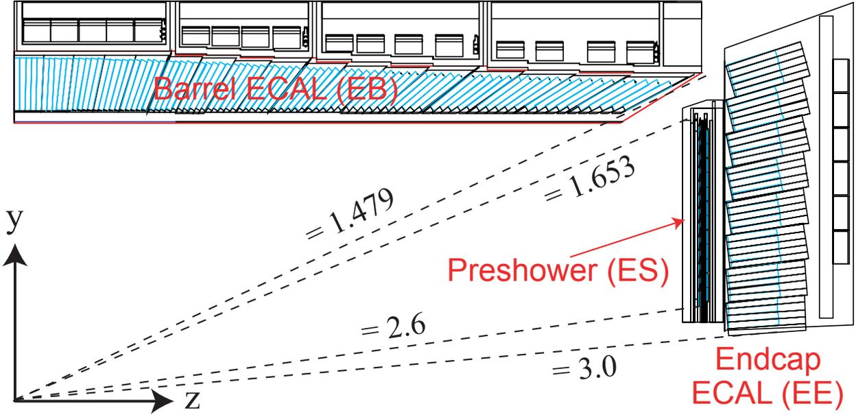
Figure 2.12: A schematic cross section of the CMS ECAL. Only one quarter of the entire ECAL is represented. The three subsystems of the ECAL: the barrel (EB), endcap (EE), and preshower (ES) are all shown. [72]
