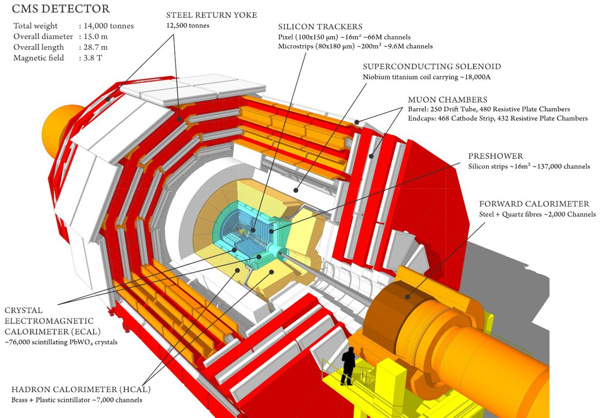
Figure 2.6: A cartoon schematic of the CMS detector
