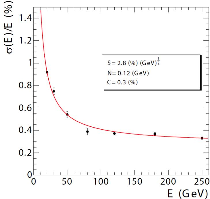
Figure 2.15: Energy resolution of the CMS ECAL as a function of electron energy as measured in a test beam. The fit (red) is parameterized by stochastic ( $S$ ), noise ( $N$ ), and constant ( $S$ ) terms, as described in Equations 2.6 and 2.7 [67].
