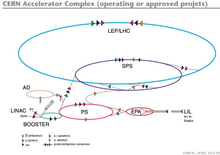
Figure 2.4: Schematic of the CERN accelerator complex [70]
