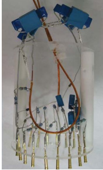
Figure 3.10: A positive high voltage divider board made of cryogenic components mounted on stress-relieved acrylic disks; the diameter of the disks is 2.5”.
