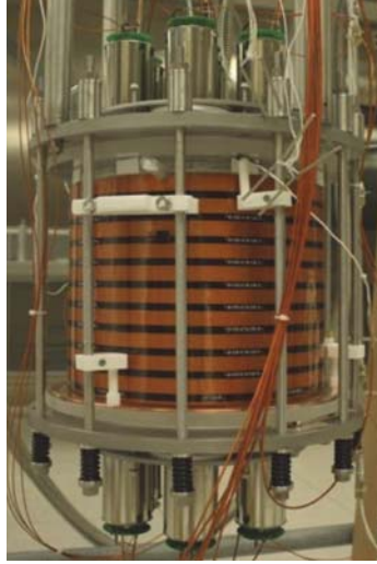
Figure 2.11: The DarkSide-10 inner detector. The sensitive argon volume is enclosed by the cylinder and seen by PMTs both from top and bottom; the black and orange strips are the field rings.
