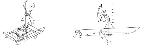
In 1981, **B.** Jöst filed for a German patent [67] (and filed for a US patent in 1984) of a propeller-driven boat that "sailed" directly against the wind, as sketched on the right above.
