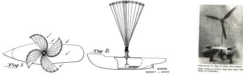
In 1960, **W. Zalewski** file a patent for a wind-propelled boat [50]. He proposed that the propeller mounting be rotatable about a vertical mast, to permit "sailing" both downwind or upwind. The figure on the right above shows a model of this from 1962 [52] (also p. 22 of [68]).
