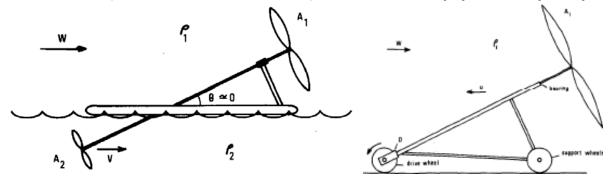
In 1980, **J.-P. Vidal** filed a patent for a propeller-driven sea yacht [65] to "sail" directly against the wind, as well as downwind faster than the wind, as sketched on the left below He claimed that this concept dates back to the 18<sup>th</sup> century, perhaps referring to the supposed Napoleonic sea "castles" [92, 98].
