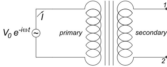
The role of the 1:1 transformer is to present a voltage drop between terminals 1 and 2 equal to the voltage drop  $V_0 e^{-i\omega t}$  of the power source. This voltage drop is equal, to a good approximation to the difference in the electric scalar potential between terminals 1 and 2 (as well as that at the terminals of the power source).
