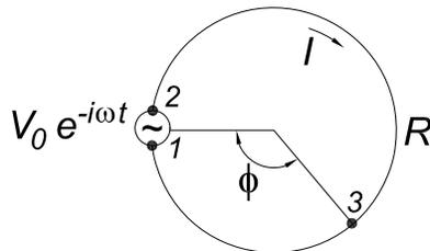
Taking the scalar potential to be zero at terminal 1 of the voltage source, and to have magnitude  $V_0$  at angle  $\phi = 2\pi - \epsilon$ , the magnitude of the scalar potential at point 3 at angle  $\phi$  is,
