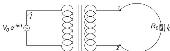
There is now a current  $I_0$  in the secondary, which is essentially uniform along the secondary loop. The coupled-circuit analysis for currents  $I$  and  $I_0$  is,
