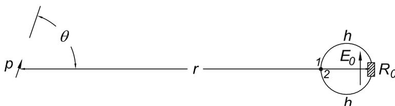
Clearly the potential difference  $V_1 - V_2$  is zero, but the meter can have a nonzero reading. We orient the loop formed by the leads such that the local electric field  $\mathbf{E}_0$  of the distant electric dipole antenna lies in the plane of the loop. Then, the magnetic field, whose magnitude is,
