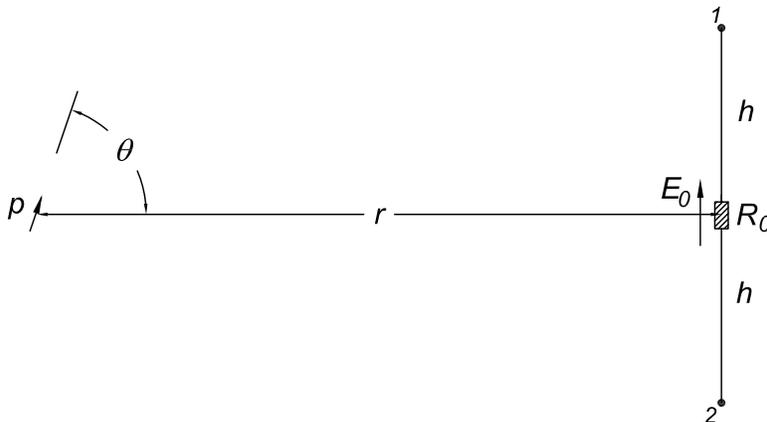
The voltmeter is in effect a dipole receiving antenna with a high resistance between its terminals. The  $\mathcal{EMF}$  across the terminals will be essentially the same as if the resistance  $R_0$  were infinite, *i.e.*, the open-circuit voltage. This voltage has been discussed elsewhere [21], and the simple result is that,
