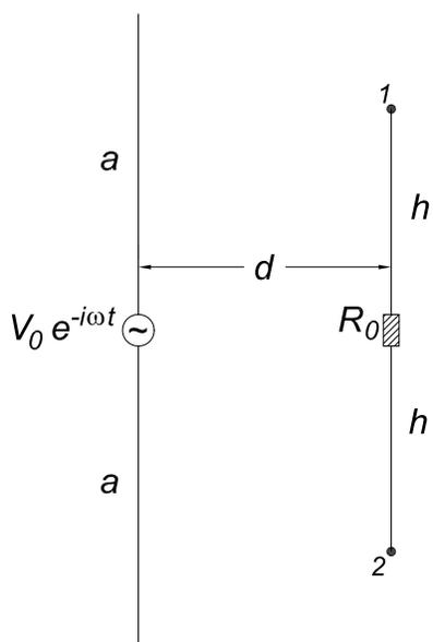
To predict the behavior of the voltmeter, I used the NEC4 simulation [23] with the LD command to generate a resistance  $R_0$  of 1 megohm. Results are given in Table 1 for a drive voltage  $V_0 = 1$  volt.
