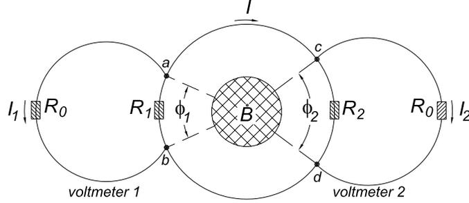
Two identical voltmeters with internal resistance  $R_0 \gg R_1, R_2$  probe the central circuit, the first connecting to points  $a$  and  $b$ , and the second connecting to points  $c$  and  $d$ . The positive leads of the voltmeters are attached to points  $a$  and  $c$ , which defines the sense of currents  $I_1$  and  $I_2$  to be as shown. We suppose that no magnetic flux from the solenoid passes through outer loops 1 and 2.
