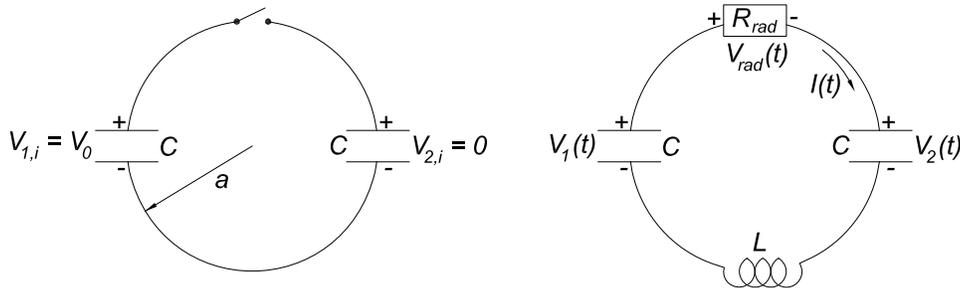
The “paradox” is that the final stored energy is  $U_f = 2(CV_f^2/2) = CV_0^2/4 = U_i/2$ , where  $U_i = CV_0^2/2$  is the initial stored energy.<sup>1</sup> Hence, half the initial energy is “missing” in the final state.
