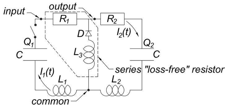
Initially,  $Q_1 = CV_0$ ,  $Q_2 = 0$ , and the switch is open, to be closed at time  $t = 0$ . The steady-state voltage and charge on the two capacitors are equal.
