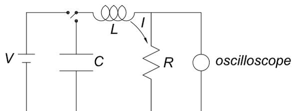
At time  $t = 0$ , a switch connected a battery of voltage  $V$  to an inductance  $L$  and resistance  $R$  in series. The voltage drop  $IR$  across the resistor was observed with an oscilloscope (of large input impedance). The current waveform corresponding to this position of the switch was,
