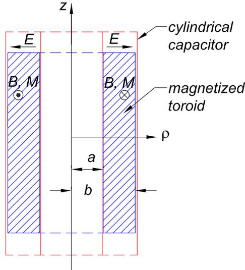
The two electrodes of the capacitor, and the toroid, can move without friction along their common axis. Ignore gravity.
