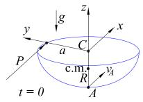
For an impulse tangent to the rim, as sketched above, the resulting angular velocity has both y- and z-components, and the subsequent motion is complex.
