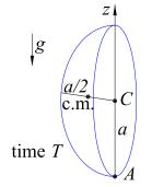
We see from the figure that the configuration of the shell when the rim touches the horizontal surface implies that the moment of inertia  $I_{z,cm}(T)$  is the same as the initial moment of inertia  $I_{y,cm}(0)$ , namely  $5ma^2/12$ . Hence,
