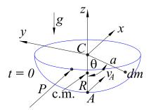
For time t > 0, after the horizontal impulse  $\mathbf{P} = p \hat{\mathbf{x}}$  at time t = 0, the only forces (ignoring friction) on the bowl are vertical: gravity and the normal force of the horizontal surface on the bowl. Hence, the horizontal velocity of the center of mass is constant for t > 0, and has value,
