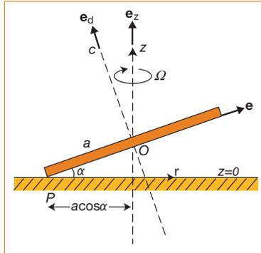
Figure 1 A heavy disk rolls on a horizontal table. The point of rolling contact  $P$  moves on a circle with angular velocity  $\Omega$ . Owing to dissipative effects, the angle  $\alpha$  decreases to zero within a finite time and  $\Omega$  increases in proportion to  $\alpha^{-1/2}$ .
