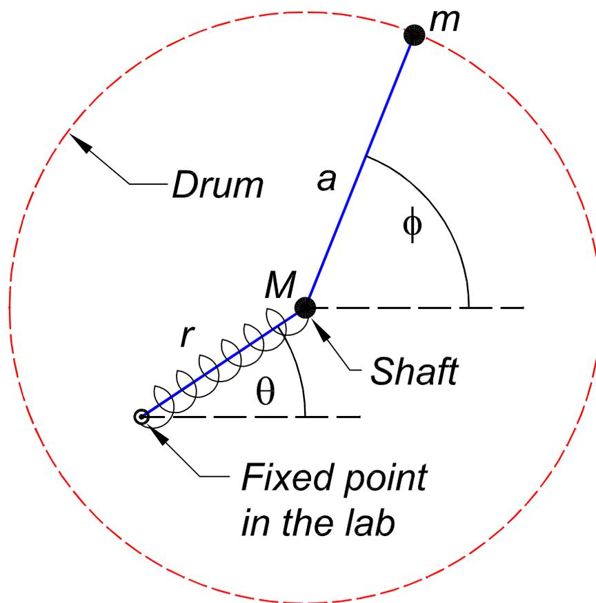
The drum and symmetrical part of the load have mass  $M$ .
