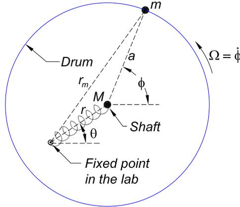
A motor forces the drum to rotate about its center with constant angular velocity  $\dot{\phi} = \Omega$ .
