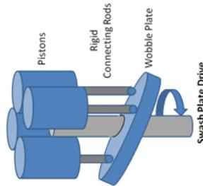
The pistons each have mass  $m$ , with their axes at distance  $r$  from the main shaft. The piston cylinders are at rest with respect to the shaft.
